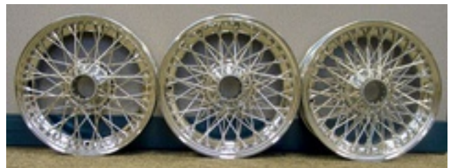
Examples of shiny new 48-spoke, 60-spoke and 72-spoke chrome and stainless wire wheels.
