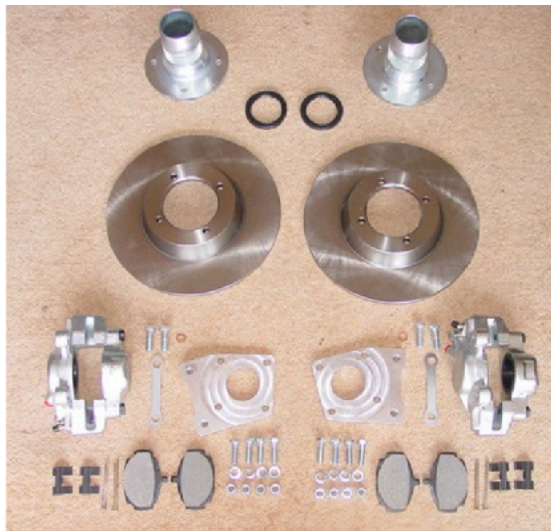
All the parts required to convert an MGA 1500 with wire wheels to front disc brakes
