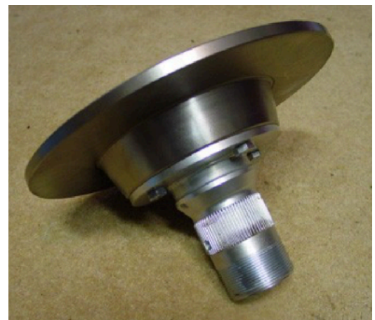
MGA 1600 brake disc and hub bolted together ready for assembly
