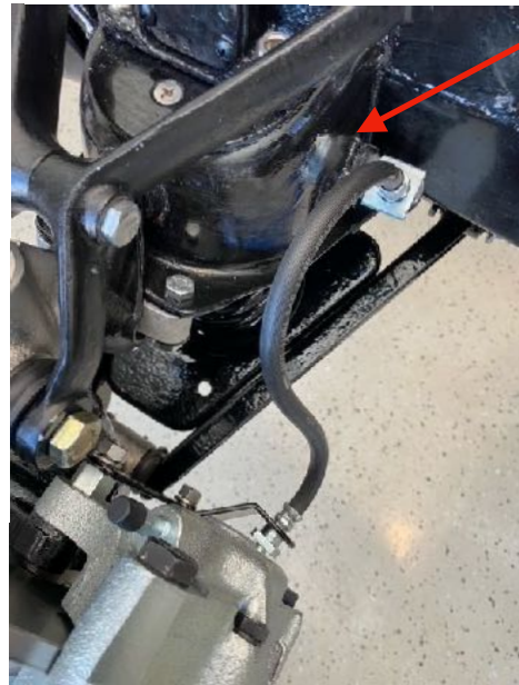
Brake hose mounting tab re-welded further back. Also need locking tab that locks hose to mount plate.
