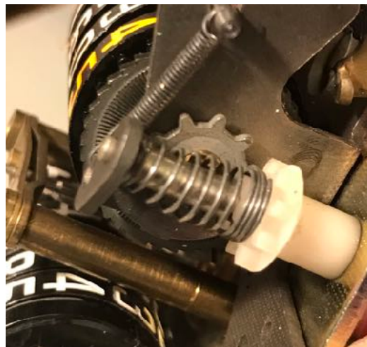
Top of reset shaft through hole in trip odometer mount. Short pin through shaft is at top of plastic gear, hidden by bottom of coarse spring.
