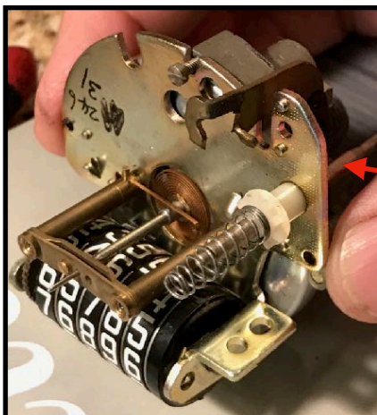
The reset shaft with coarse spring and plastic gear over it after the trip odometer is removed. When putting trip odometer back together, this shaft must be put back in place first with gear and spring. Note fine hairspring also.
