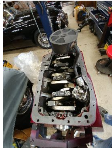
Allan Bachelder's mounting plate to mount the Magnette pan on the MGB engine
