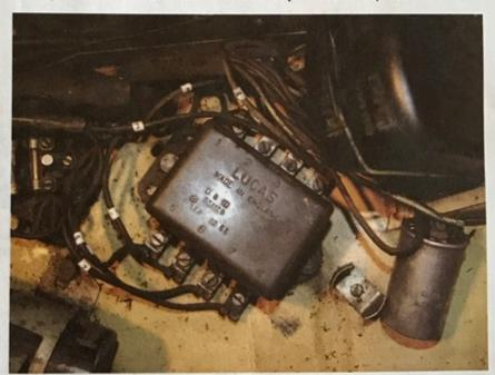
Though the Lucas switch did not function properly, it was not the reason that the blinkers and brake lights stopped working. The problem was in this Lucas relay mounted on the firewall.
