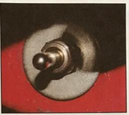
We also replaced the brake light switch (the screwin type with two terminals with screw-in connectors) with a store-bought Standard Auto Parts switch and then we installed this toggle switch. It also worked perfectly.
