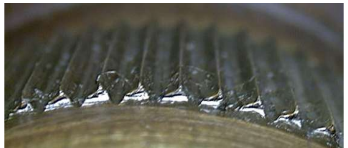
Bad: Hub spline very badly worn - skewed flank and sharp apex.
