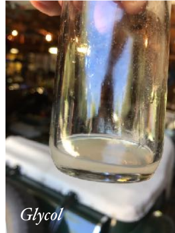
Jar on Left has Glycol brake fluid mixed with water.
