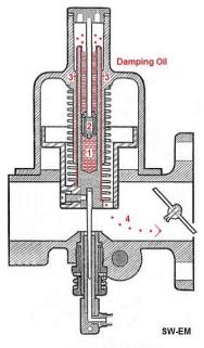
holes in bottom of Dashpot)" This explains the slow loss of damping oil and the need to occasionally replenish it.
