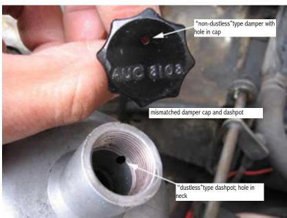
**mismatched** - vented "non-dustless" damper cap and vented "dustless" dashpot-note the smooth neck of the air chamber body on this SU carb
