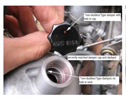
**matched** - vented "non-dustless" damper cap and unvented "non-dustless" dashpot-note the shoulder on the neck of the air chamber body.
