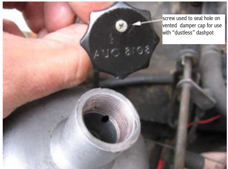
fixed - "non-dustless" damper with vent sealed, and vented "dustless" dashpot
