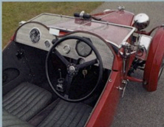
The twin-hump cowl ("scuttle" in Brit-speak) and folding windshield debuted on the rakish J2, and became beloved MG roadster styling cues.
