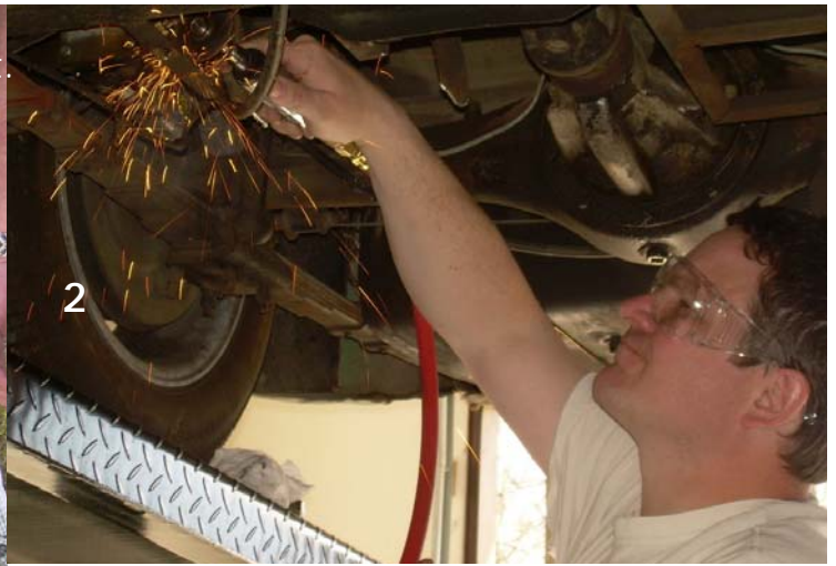
1) Rob and Neil discuss the best approach to attach a new battery support bracket in Matt Wigent's MGA with Rob's new MIG welder. 2) Sparks fly as Matt cuts out the old rusted battery frame. 3) Rob, Mike, Brian & Matt watch as Neil finishes the installation. 4) Neil makes one last check to inspect his work before handing it over to Matt. 5) Gordie, Mike, Steve & Cathy enjoy hanging out in the sunshine for a change. 6) The full view of Rob's '37 Ford chopper. This one ought to keep him busy for a while.
