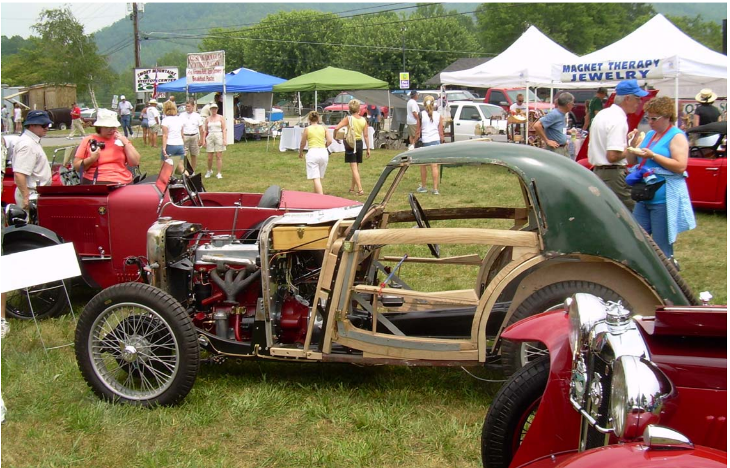
A 1930's era MG Airline Coupe in restoration at the MG 2006 GT in Gatlinburg. Note the extensive wood framing.
