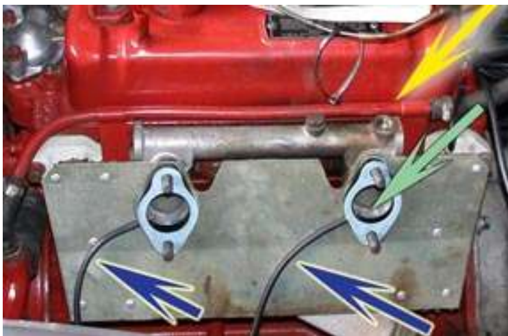
Picture No.4 Close Up Of Installation to Carbie Distance Blocks
