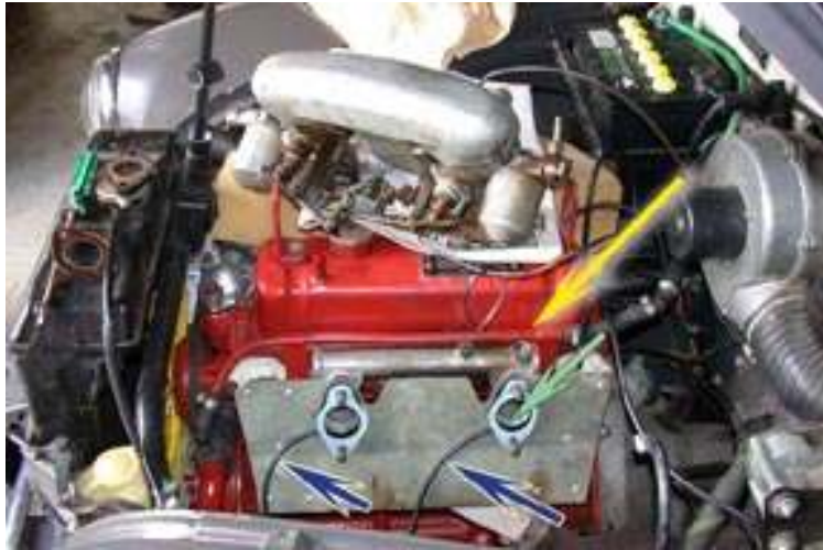
Picture No.3 Vacuum Tubing Installation at Manifold
