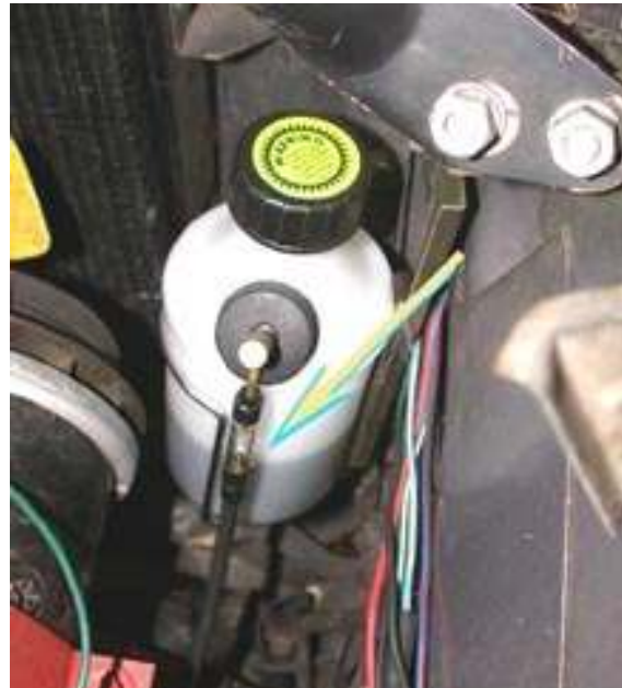
Picture No1 Sight Glass Highlighted.
