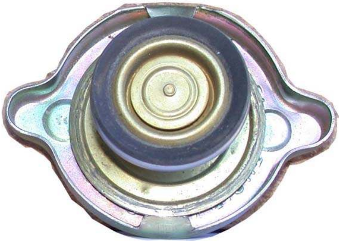
Picture 3b End View – Standard 50's Radiator Cap. Note vacuum relief valve at centre
