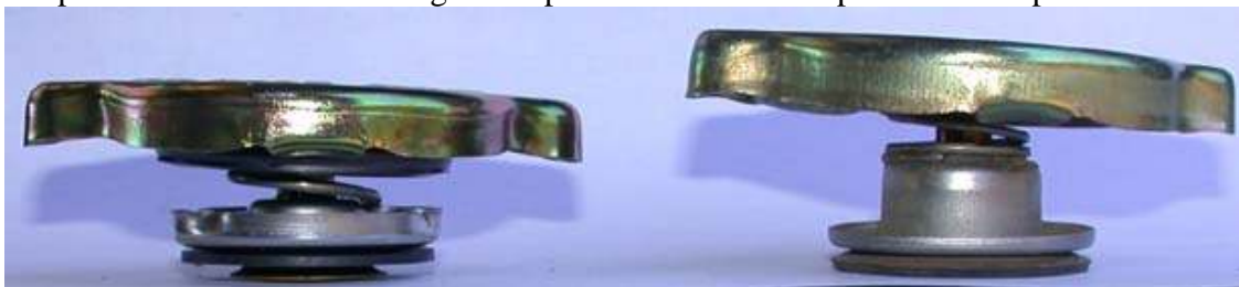
Picture 2 Radiator Caps - Recovery type left and standard 1950's type right
