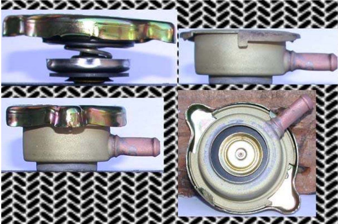
Picture 9. Radiator Housing with Recovery Cap installed – Side and End view
