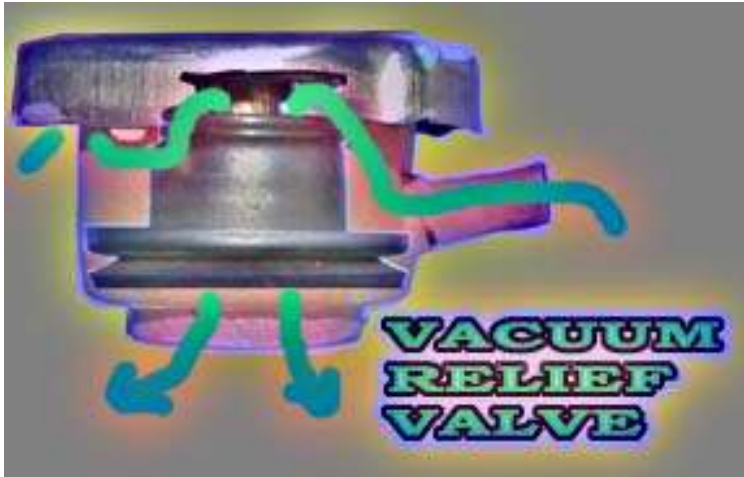
Picture 5. Radiator goes cold and relief valve sucked open.
