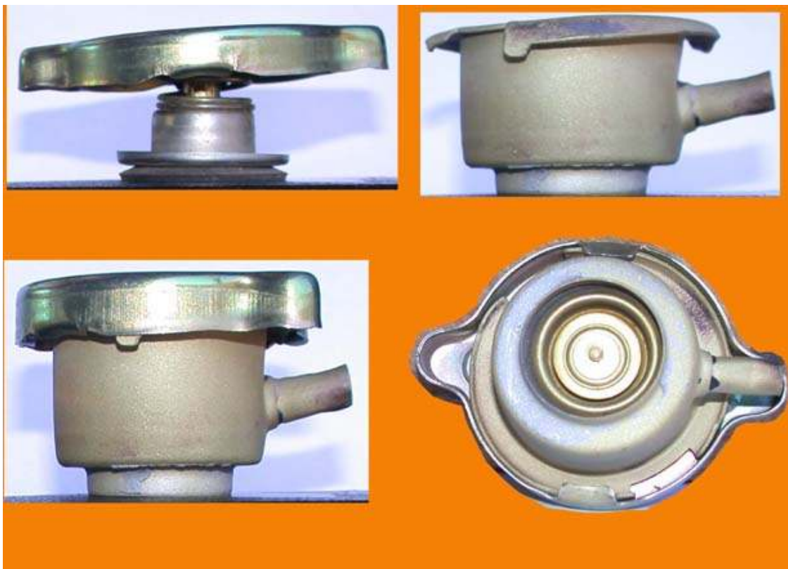
Picture 6. 1950's Radiator Housing with Cap installed – Side and End view
