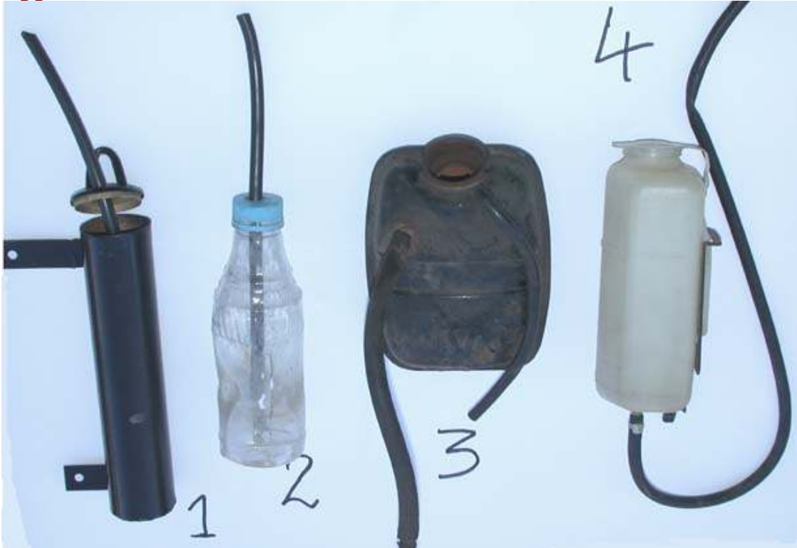
Picture 10. Four types of expansion containers
