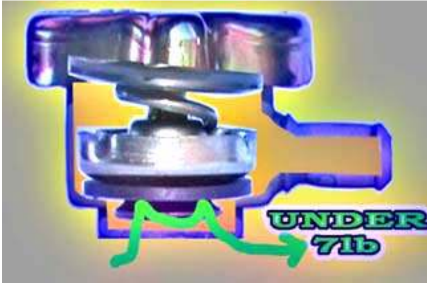
Picture 8a. Internal pressure less than 7 lb.
