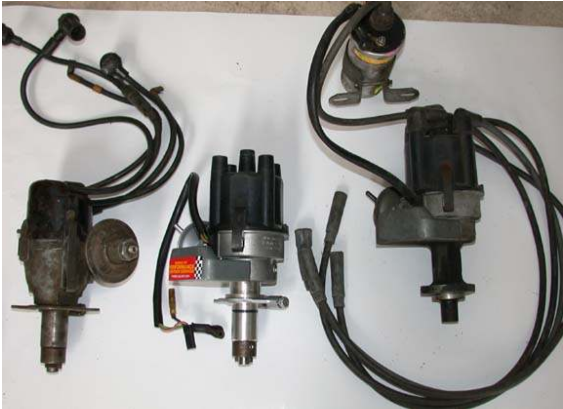
Picture 3. Comparison: DM2, Modified & Unmodified Electronic Bosch Dizzy
