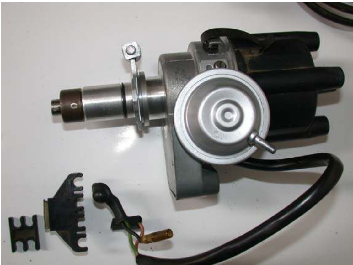
Picture 4. Modified Bosch 9230 064 519 Electronic Distributor
