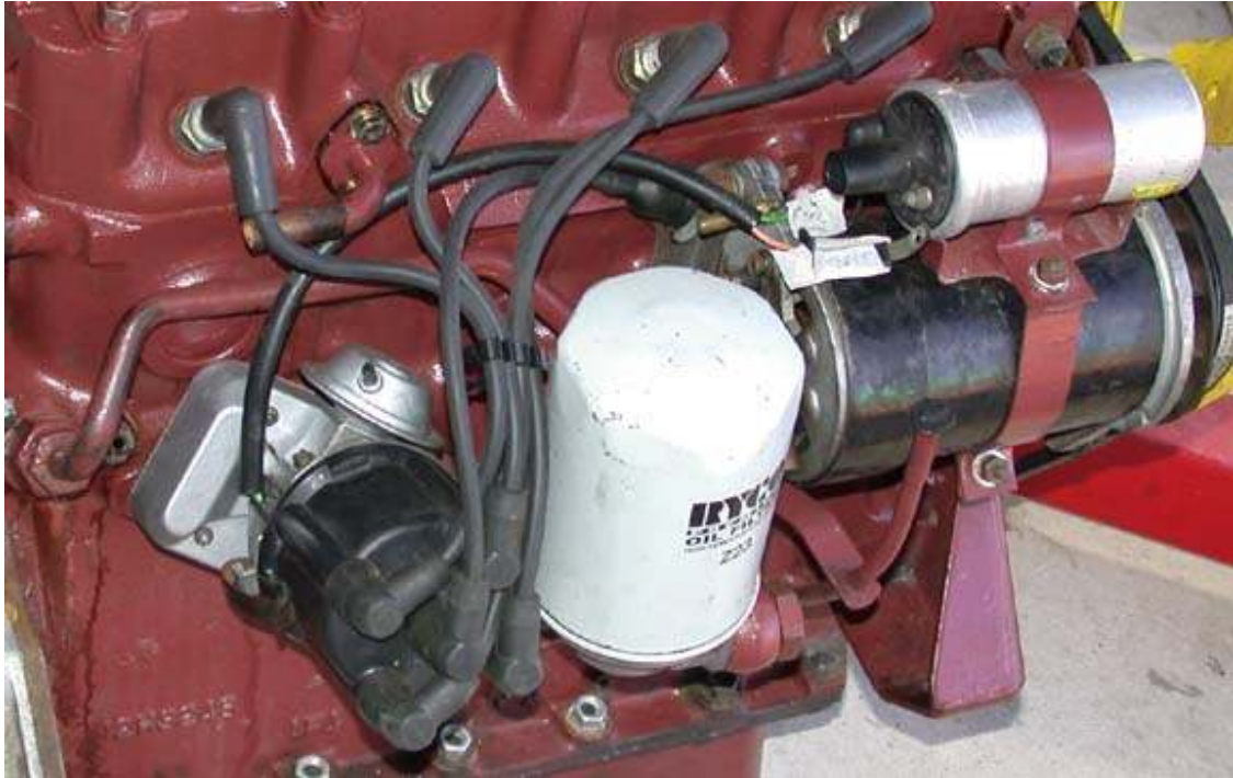
Picture 2. Modified distributor installed.
