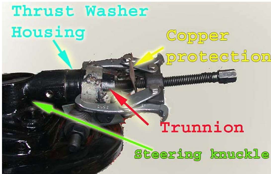
Picture 7. Clamp and puller used to release the upper trunnion
