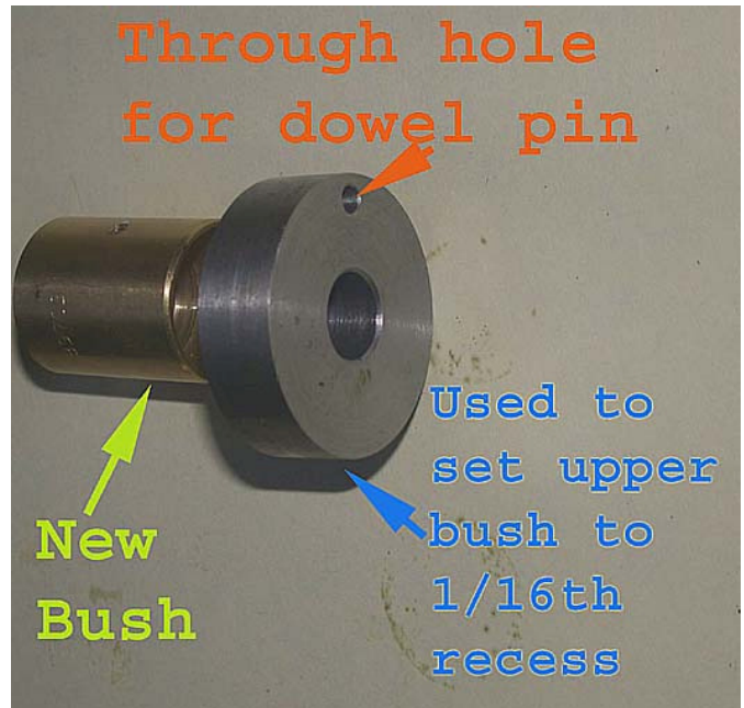
Picture 6b. Gauge used for correctly recessing the upper bush
