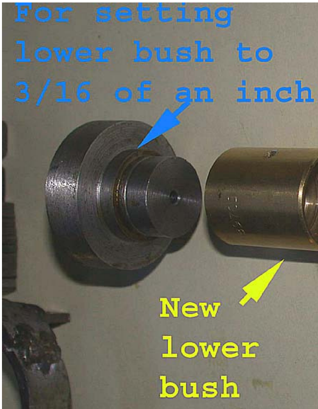
Picture 6a. Gauge correctly recesses lower bush
