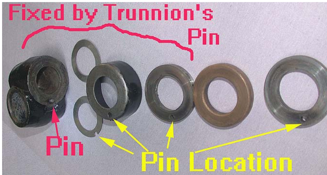
Picture 3. Trunnion Assembly: Trunnion, shims & housing [with thrust washers]
