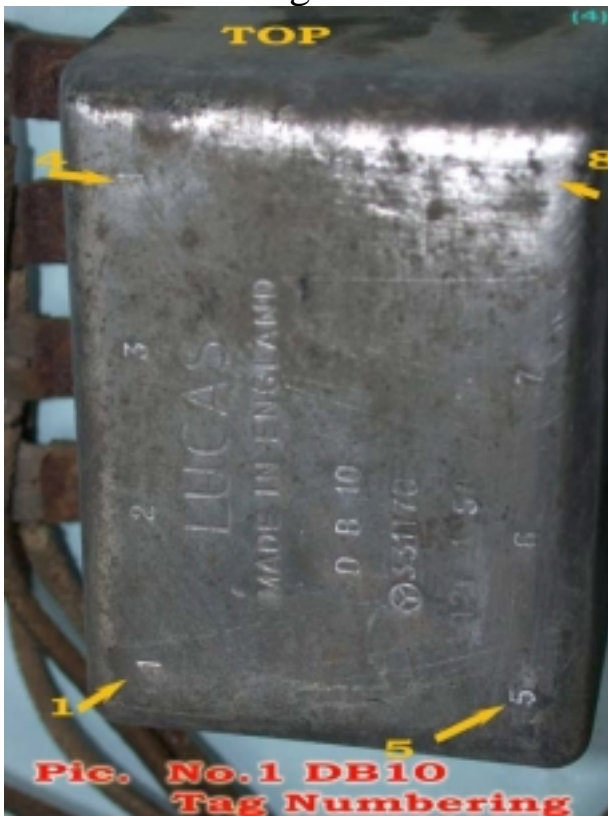
Picture 1. Wire Termination [Tag] Numbering
