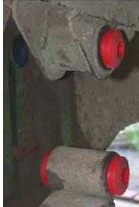
Pic4. Initial installation of new 'Ford' bushes
