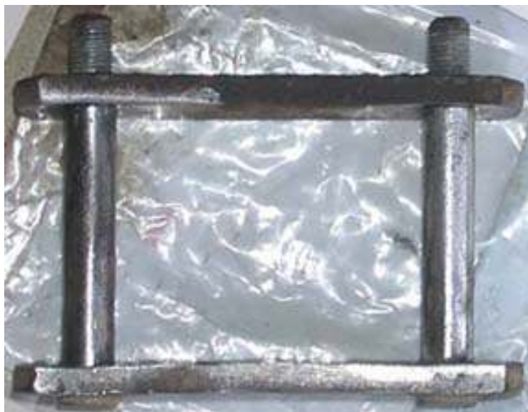
Pic3. Original MG Magnette shackle polished in preparation for installation
