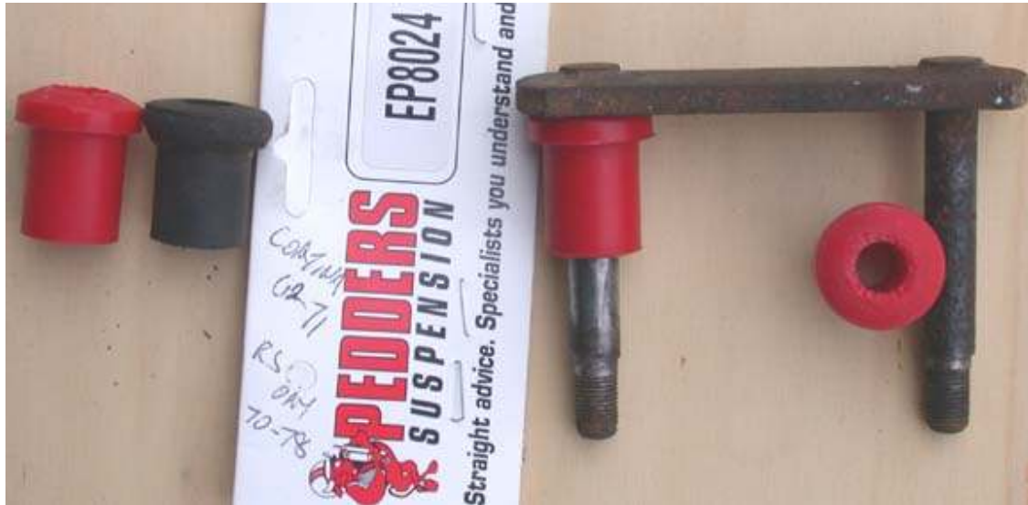
Pic2. Original MG ZA/ZB shackle [rusty]. Replacement ‘Ford – EP8024’ bush with modified head, but not yet cut to length, is compared to used rubber original
