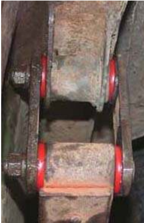
Pic6. New 'Ford' bushes in place – Rear view
