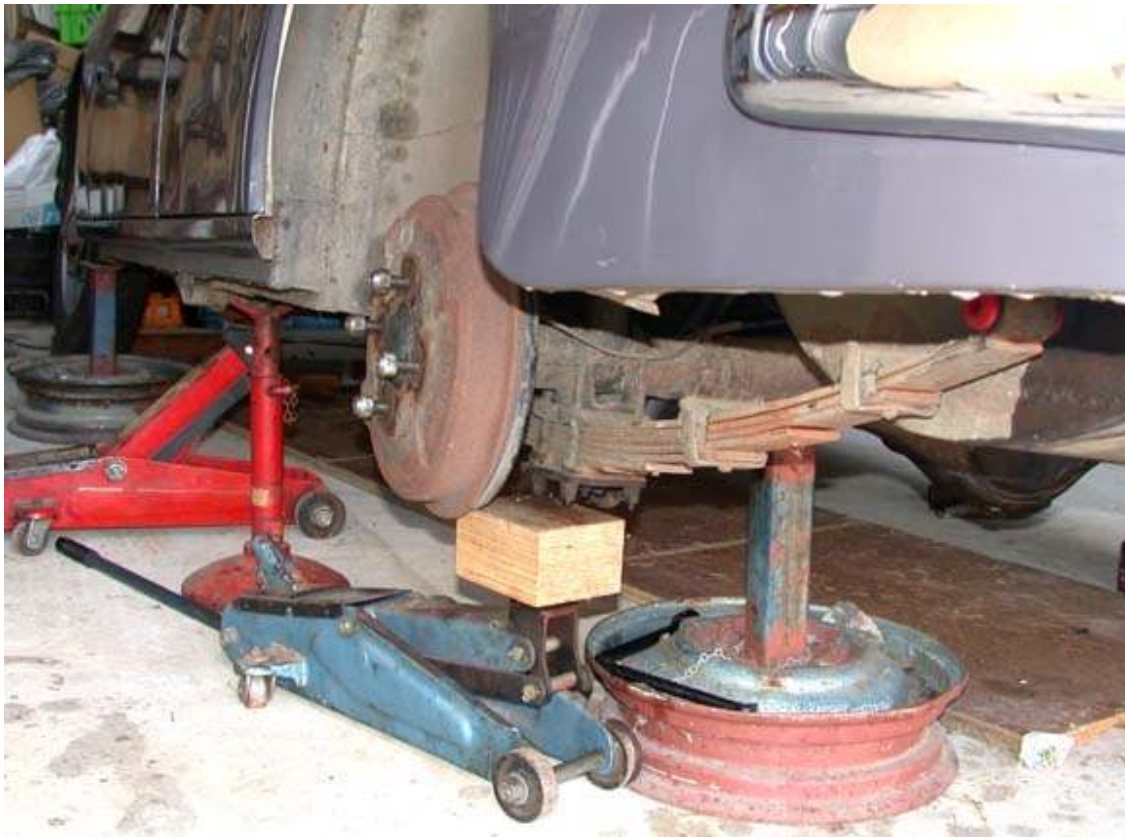
Pic5. Jacking: Two body safety stands, one axle safety stand, one body jack and one axle jack
