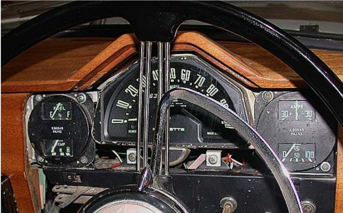
Picture No 7 Updated temperature gauge and its cluster reinstalled [four screws]
