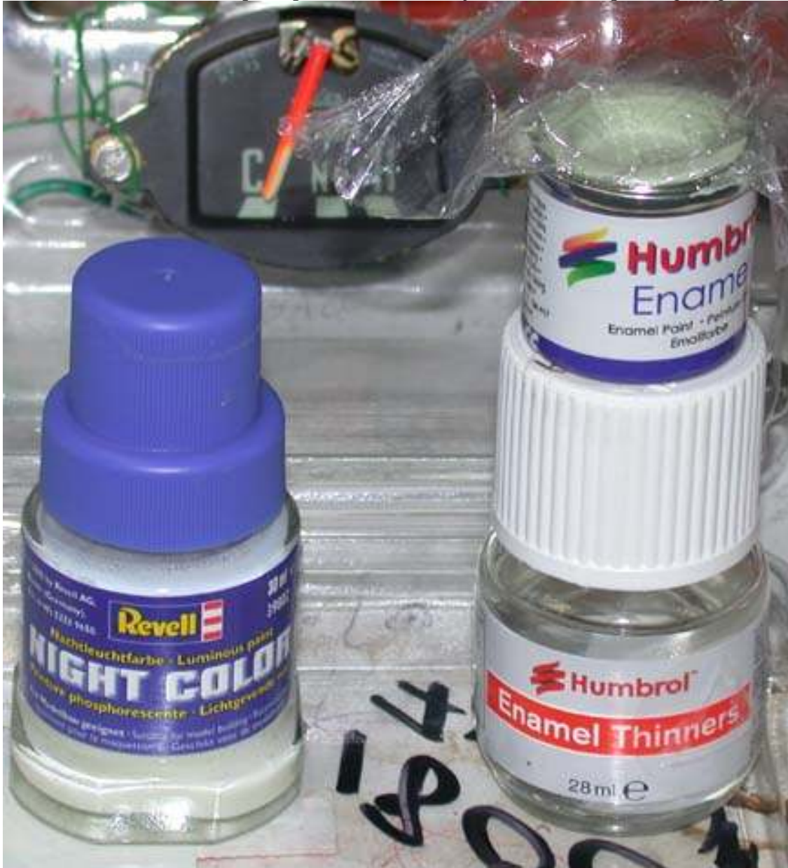
Picture No 6 Enamel and luminous paint for the pointer.
