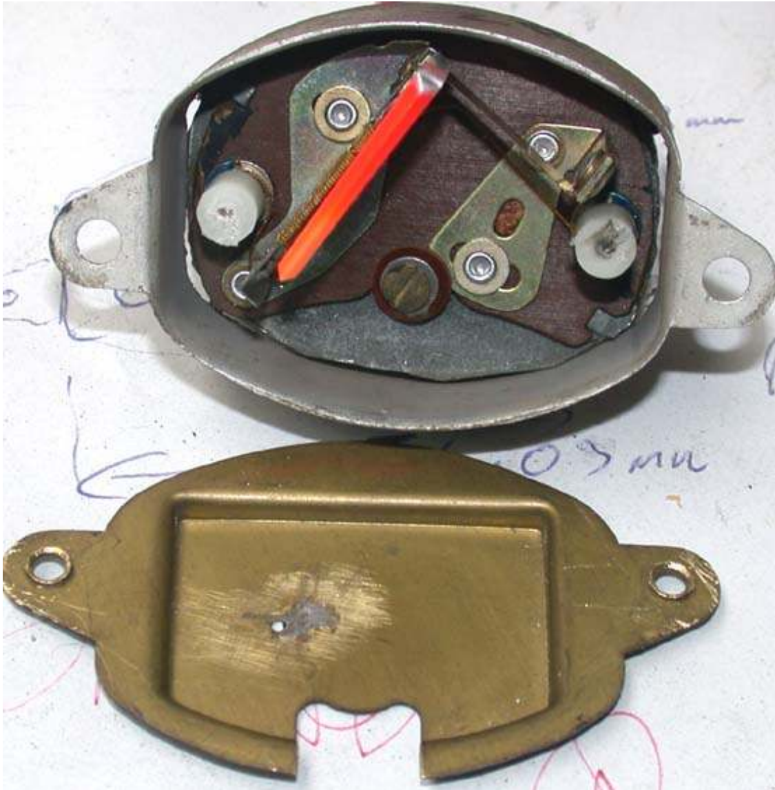
Picture No 5 New internals fitted and retained with two bolts and silicon sealer
