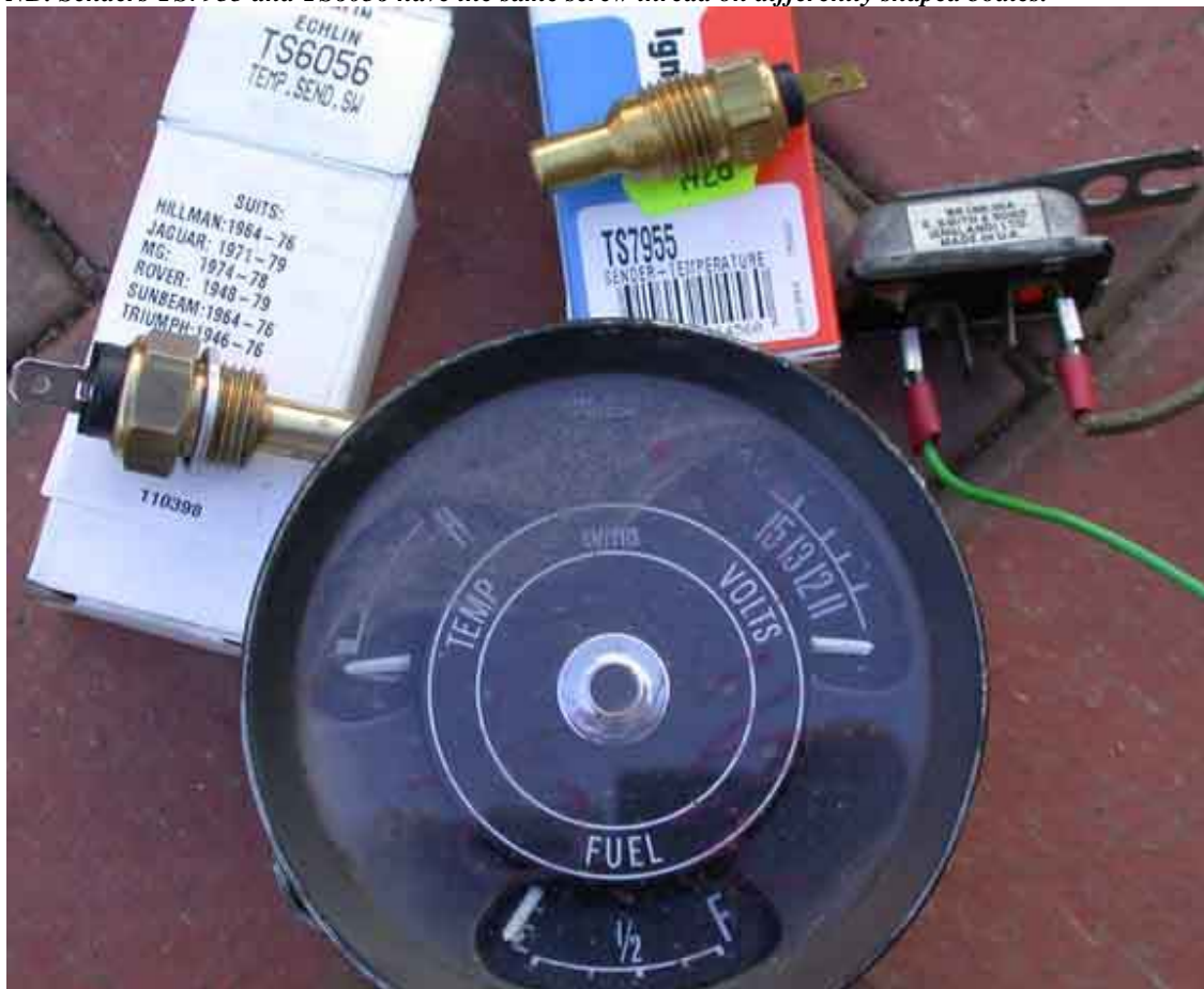
Picture 1 Temp senders, Voltage stabilizer and Triumph instrument cluster
