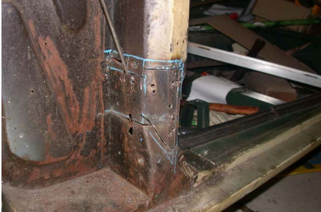
Figure 2 Lower A Pillar – Part outer skin being released from spot welds to access rusted carrier
