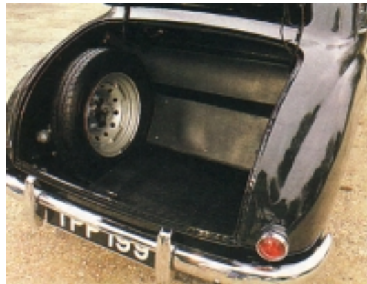
Vertically-mounted spare wheel shows depth of roomy boot, which has low loading height.
