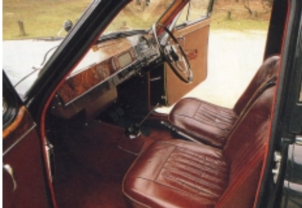
Early ZA models have a metal top dash, grained to look like wood. Leather restorer has been used on the seats.
