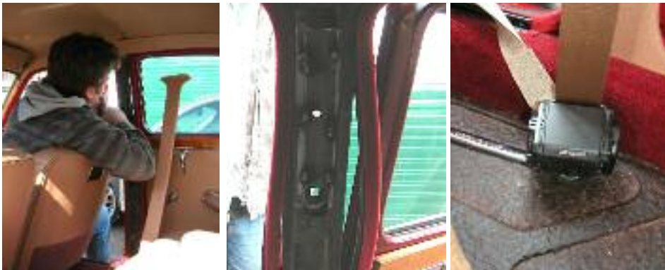
Above: As we were about to take the ZA on a continental holiday, the car was booked into Chisbon Restorations to have front seat belts fitted. Adrian had to make up special metal plates (right) for the anchor points under floor and transition. He used, and strengthened, the old semaphore point for the top belt mountings
