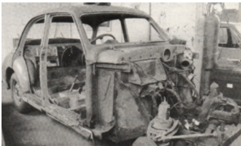
Above, stripping down the Midget was the easy part of the restoration saga.
