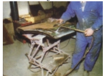
Above, repair sections were welded into the doors and joints lead loaded flush.
