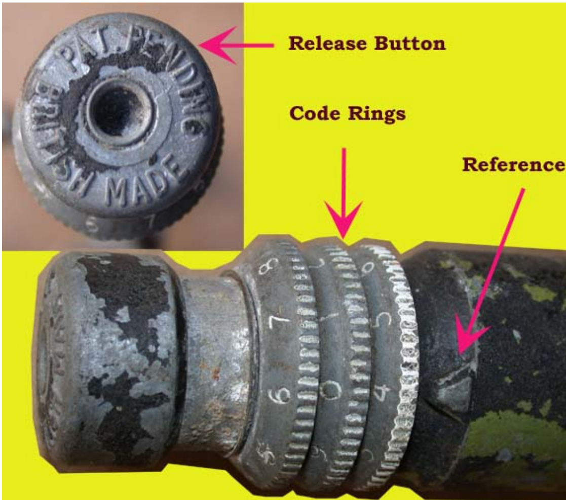
Picture 3. Close up of Reference, Dial [Code] Rings and Labeling
