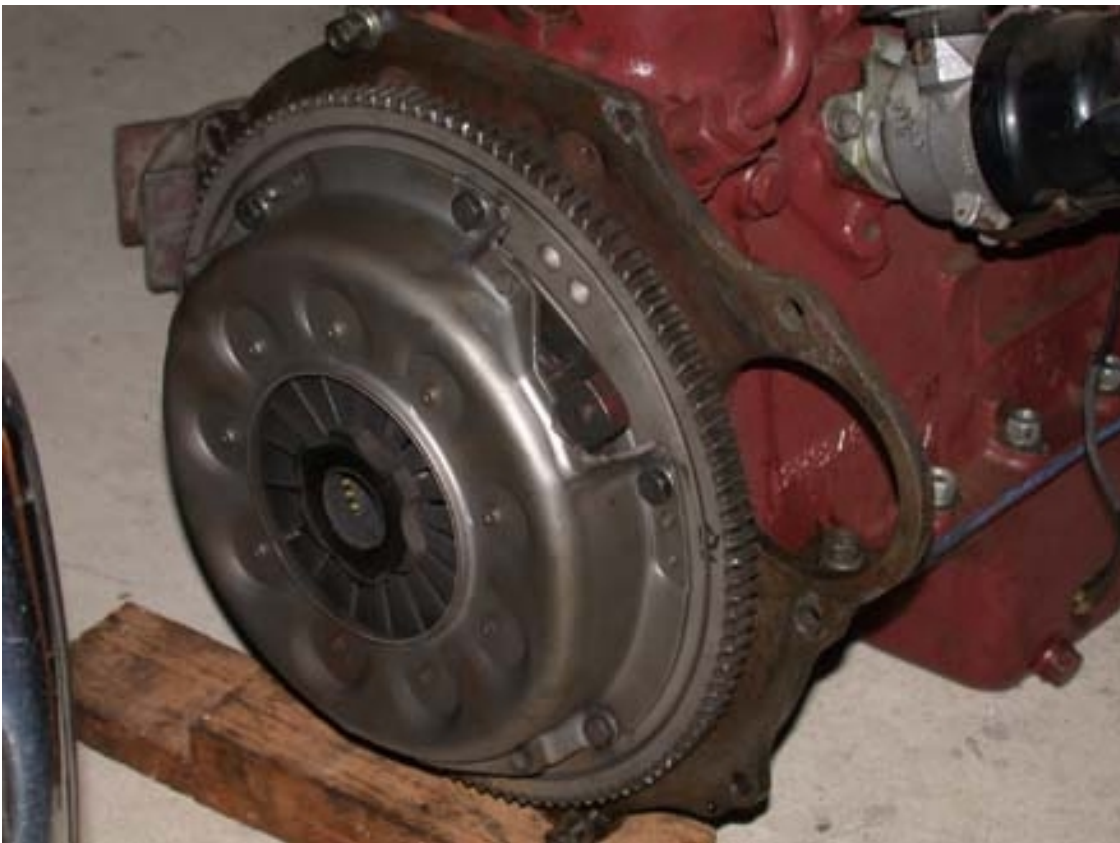
Picture one- Standard Backplate for Z Type with MGB/Austin1800 Fly Wheel & MGB Clutch Pressure Plate
