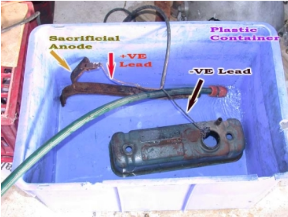
Picture No4. Cover items in tap water [With 12v battery charger turned off]
