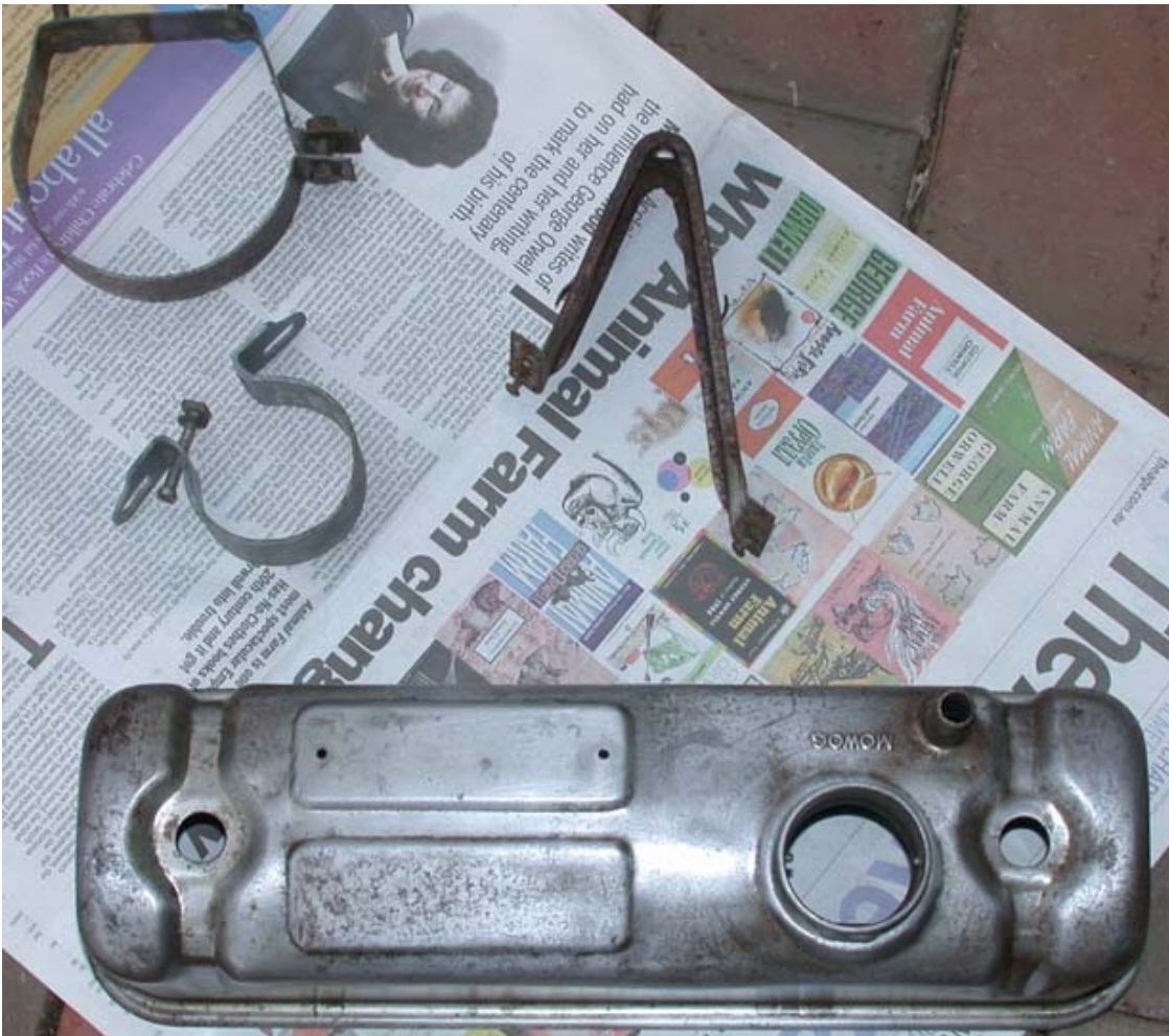
Picture 9. Final stage – All parts cleaned in caustic bath [Don't look we're exposed!] NB- Tappet cover needed two dips and small amount of paint stripper to look this good.
