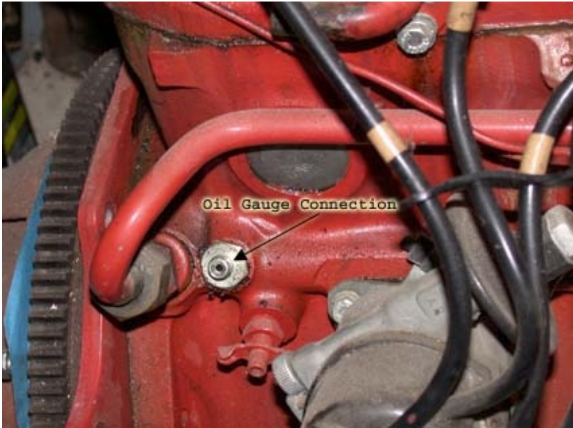
Picture 2. OIL PRESSURE GAUGE - ACCESS POINT
