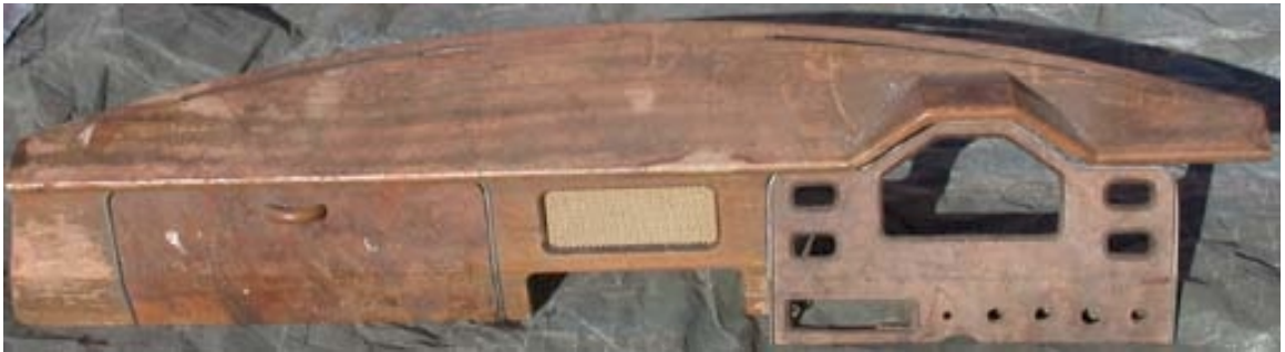
Fig3a. Shown is the dashboard in its un-restored state. Note. Instrument panel is included as an example of potential mismatch.
