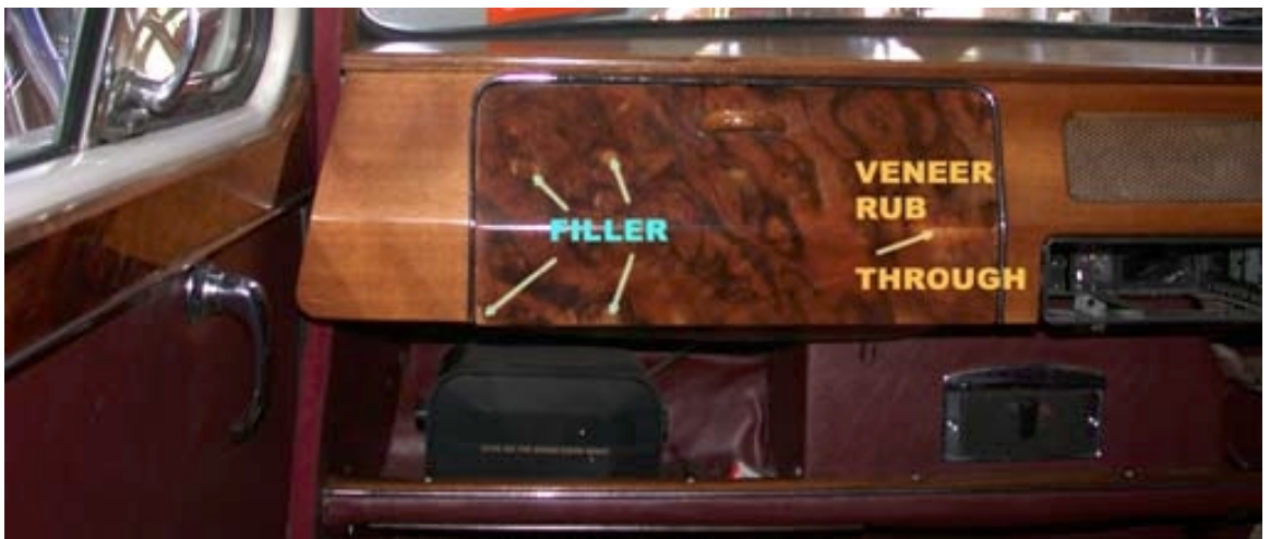
Fig 4. Partial picture of dashboard and door capping with indicated blemish and repairs.
