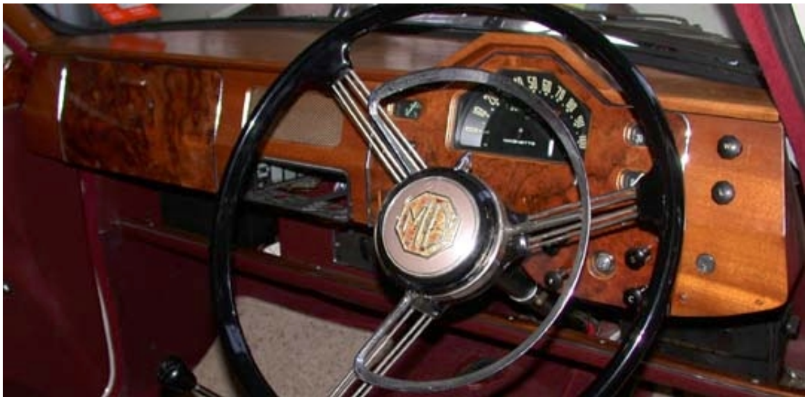
Fig 2. ZB shown here has the full mix of veneers and solid wood {Chrome borders enhance the instrument cluster, glove box & parcel shelf}
