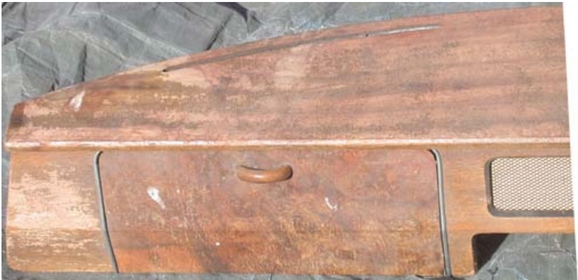
Fig3b. Close up of dashboard woodwork to be restored {solid wood on top and two veneer types on the front}
