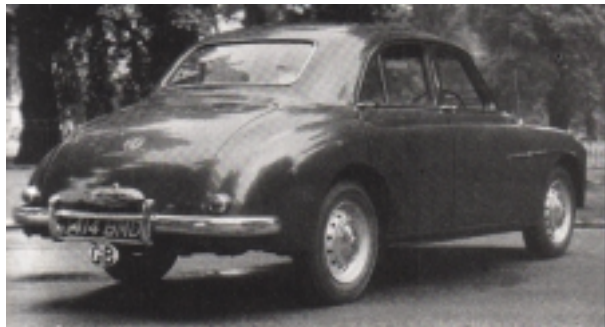
The original ZA-note small back window and chrome strip sweeping over the front wheel arch
