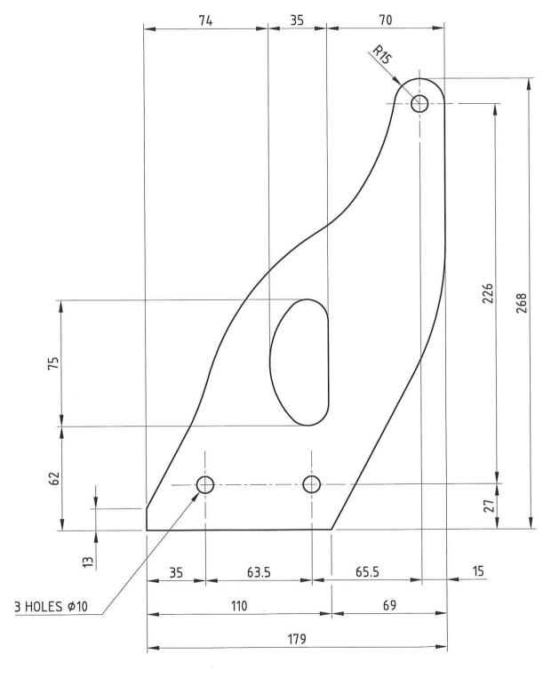
This template is designed to suit the ride height and axle location of my car. It also required modification to the bump stops and available extension of the telescopic shock absorber I used. Richard Prior
