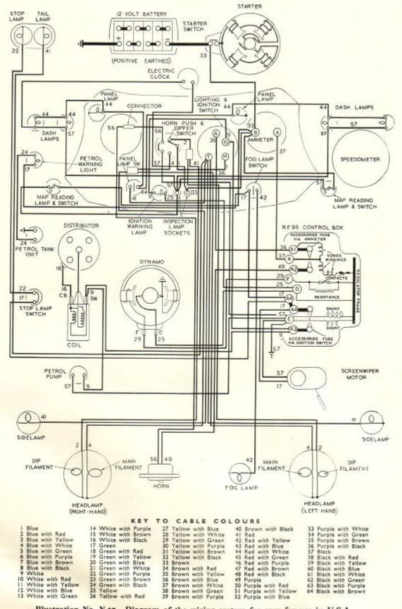
Illustration No. N.27. Diagram of the wiring system for cars for use in U.S.A.
