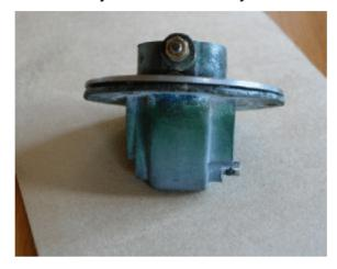
may penetrate the gasket which expands. This causes the flange to distort between the machine screws. Petrol can now seep past the gasket. A common answer is to fit a slightly thicker gasket to take up the distortion. However, the softness of the Mazak will result in further distortion of the
