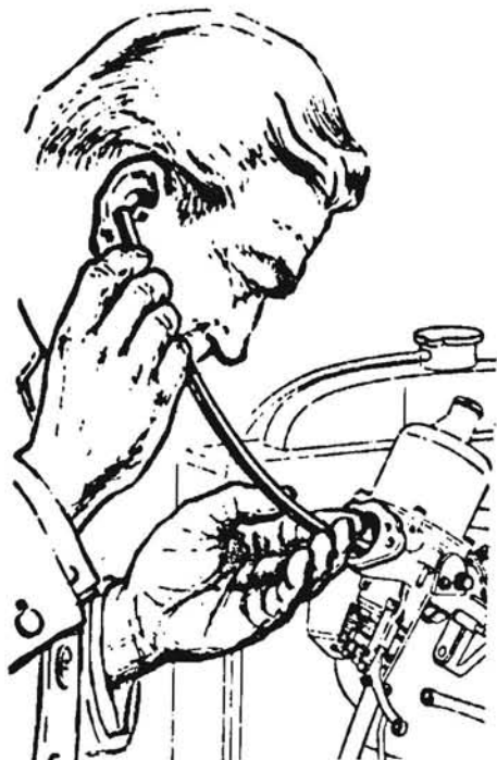
Fig. 16: Synchronization may be tested using rubber tube as stethoscope, but Uni-Syn is more accurate.
