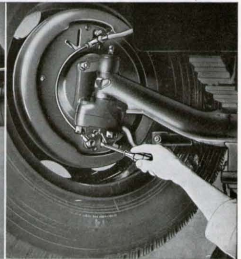
Fig. 37 Adjusting front brake shoes
