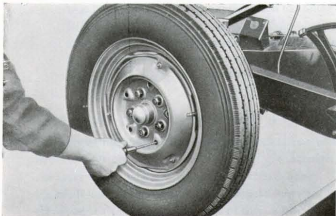
Fig. 4. Adjusting front brake shoes.
