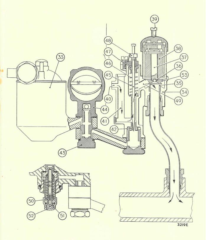
The device is brought into action by energizing the winding of the solenoid (38) from the terminal screws (39). The centrally located iron core (37) is thus raised magnetically, carrying with it the ball-jointed disc valve (36) against the load of the small conical spring (53) and thus uncovering the aperture provided by the seating (35).
