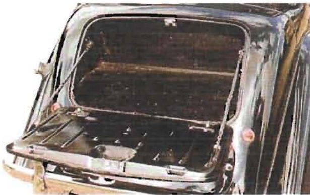
Boot space is limited, but additional luggage can be carried on the boot lid
