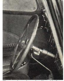
The steering column is adjustable for a 3 in. movement, and the 16 in. diameter wheel is spring spoked. Steering is by a rack and pinion type gear which is light and positive.
