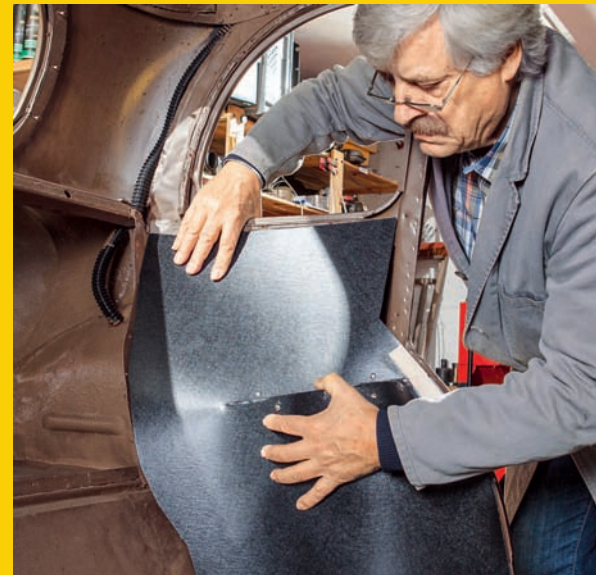
Most of the interior trim was missing. Walter cuts reinforced cardboard to measure
