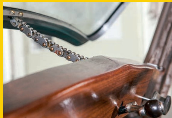
Air conditioning, pre-war style: The windscreen can be cracked open by pulling a chain - and for those wind-in-the-hair types, there's always the sunroof...
