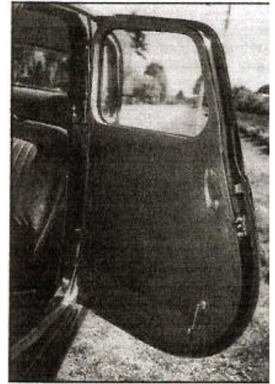
(Above) Suicide front doors, and the window winders you are just not supposed to be able to reach without honking the horn with your nose!
