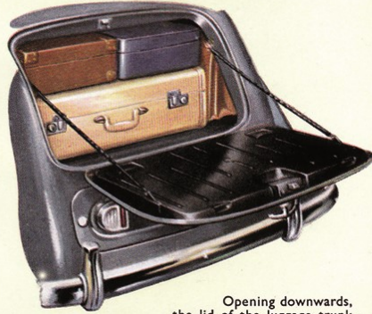
Opening downwards, the lid of the luggage trunk forms an additional luggage carrier. The general appearance of the M.G. Series "YB" Saloon has been
