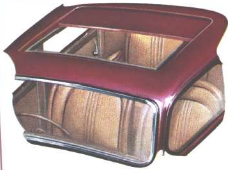
A sliding panel is fitted flush with the roof. It is skilfully designed to ensure that, when in the open position, rear passengers are free from draught. Above the driver's head is a switch which operates the roof light.
