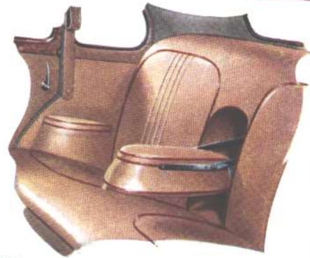
Finest grade English leather is used for the upholstery. Pleating in seats and squabs gives a very pleasing effect. The wide arm-rest for the rear seats folds back flush with the rear squab.
