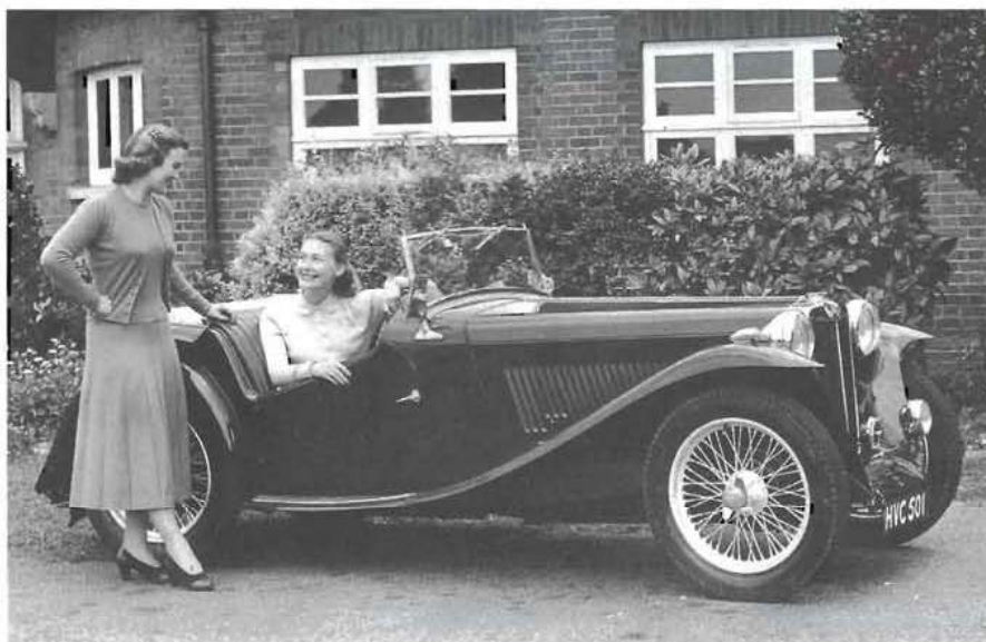
Sweet, picturesque but old fashioned: the TC of 1945 with old-style beam front axle.
