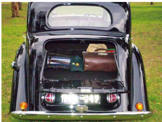
Above: Boot can take a suitcase (just), or four Gladstone bags – the fold-down lid was strong enough to support luggage.
