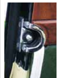
Above: The door locks just as if they had emerged from the factory. Note the seal channel, taken from a scrapped door and attached to this one. >
