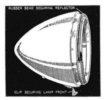
Reflector secured by rubber bead.
