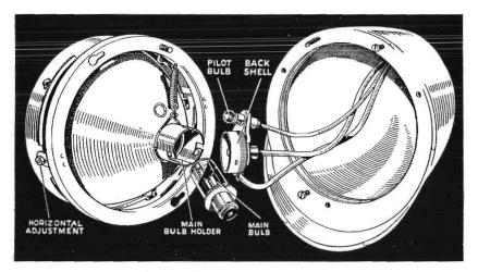
Flush-Fitting Headlamp with Light Unit removed.
