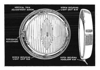
Flush-Fitting Headlamp, with Front Rim Removed.
