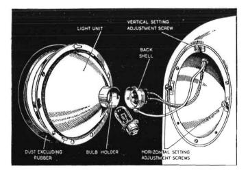
Flush Fitting Headlamp, Mark II, with Light Unit Removed.
