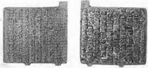
OVERCHARGED NEGATIVE & POSITIVE PLATES
