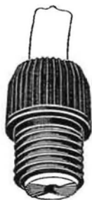
Fig. 9. METHOD OF FITTING CABLE TERMINALS.
