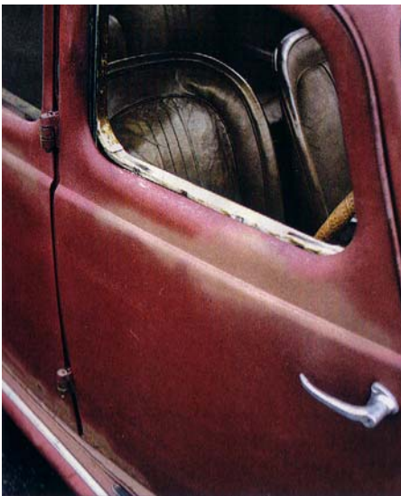
Weathered paint and worn weatherstrip show where driver's arm tends to rest
