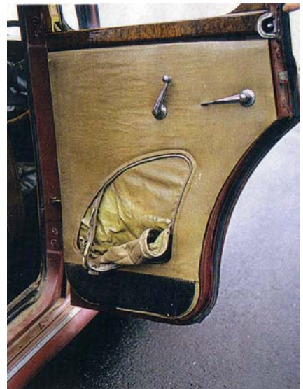
Stitching on pocket has failed but door panel belies its 50-plus years
