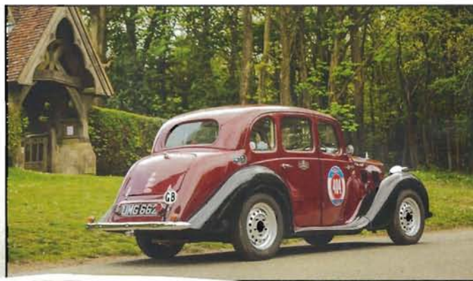
Flashing indicators replace the trafficators, for safety reasons. YBs have 15in wheels rather than the 16in rims of the YA
