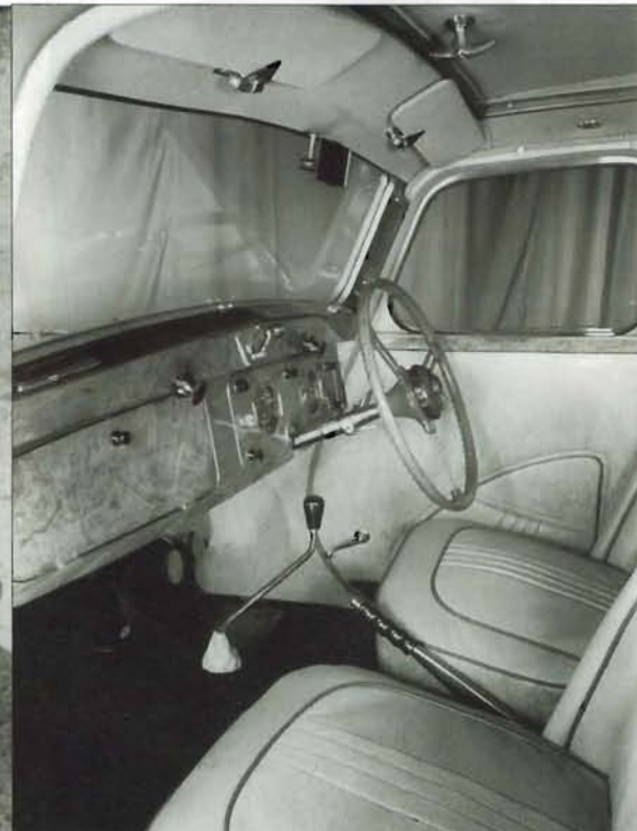
The appeal of the Y-type cabin can be seen in this picture. There are twin sun visors, a sun roof, polished wood dashboard with a glove locker, the windscreen can be opened outwards to increase ventilation and the cranked gear lever and central handbrake lever are well placed for the keen driver
