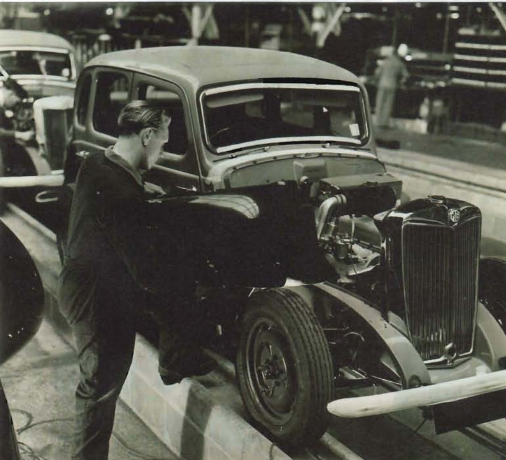
A Y-type saloon nearing completion on the Abingdon assembly lines. This car had a two-colour paint finish and the operator is fitting the darker colour wings to the body that is finished in a lighter shade
