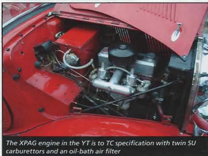
The neat engine compartment. The unit to the right of the scuttle operates the built-in jacking system
