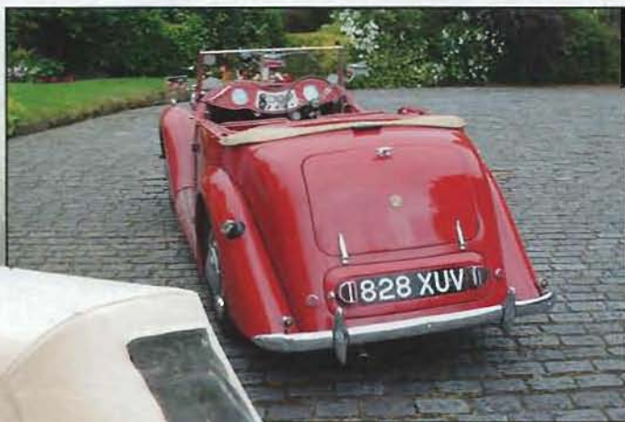
The rear section of the YT body is almost the same as that on the saloon. The spare wheel fits in the compartment behind the number plate
