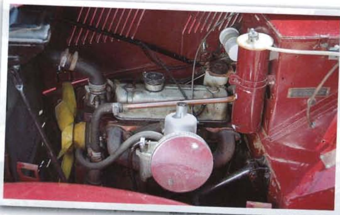
Yes, it's a good old A-Series 1275cc engine from a Marina. It provides a bit more zip than the standard XPAG unit.
