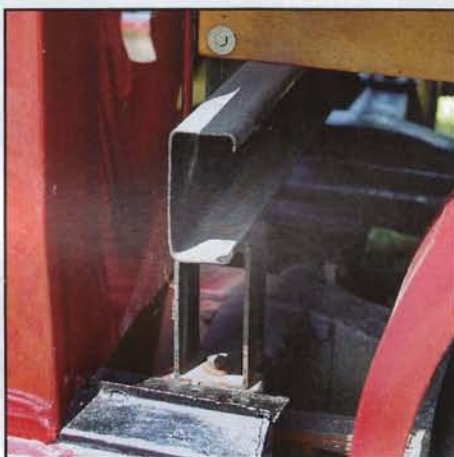
The front end of the loadbed is extremely well supported.
